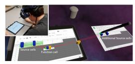
Figure 4: Neighboring sheets can also be accessed via in-air pointing. Here, the user extends the contribution to a function he defines, adding a cell of a neighboring sheet.
